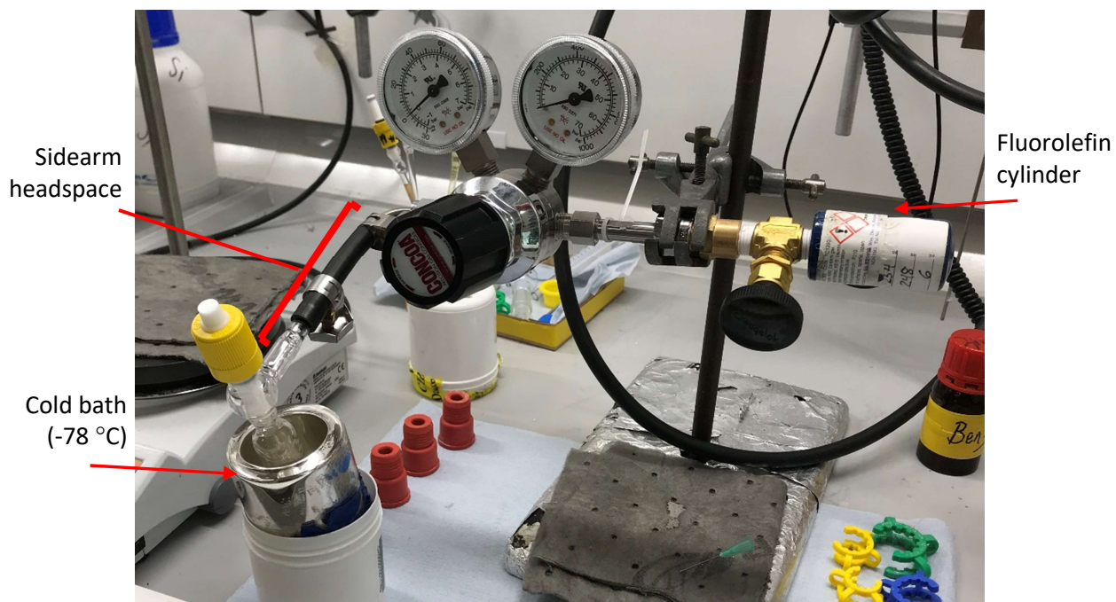
Figure 3.20 Standard set-up for large scale reactions of fluoroolefins at -78 °C
