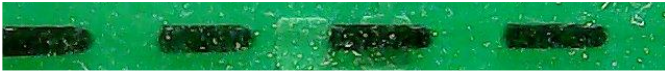
Fig.14. A typical case in monitoring experiments (the dispersed phase flow rate and continuous flow rate are all 500 \mu\text{L/h} )
