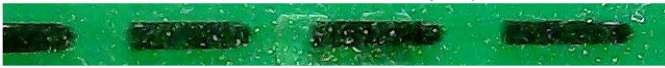
Fig.15. A typical case in monitoring experiments (the dispersed phase flow rate and continuous flow rate are all 700 \mu\text{L/h} and 500 \mu\text{L/h} , respectively).
