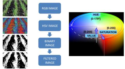
Fig. 4. Workflow of leaf area calculation method.
