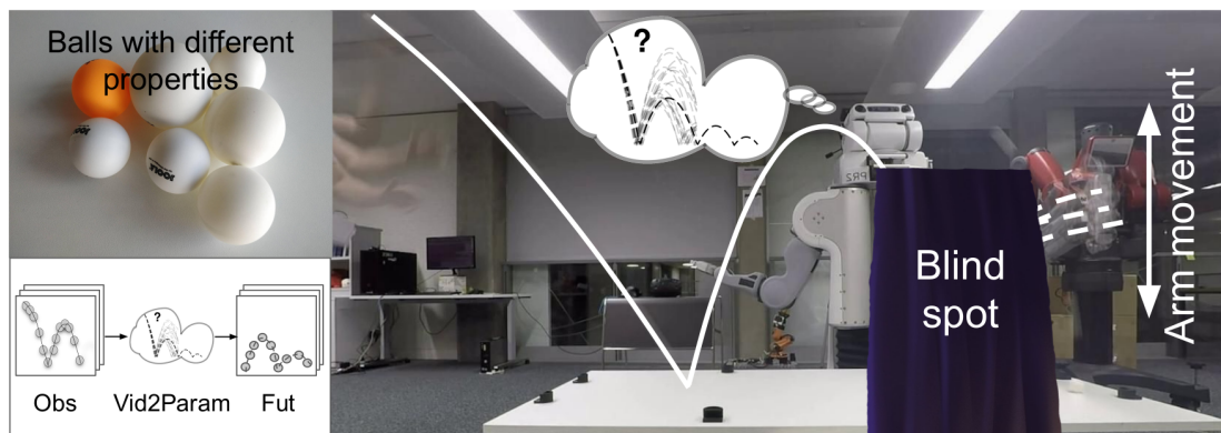
Figure 5.1: Overview and experimental setup. We are interested in reasoning about the dynamics in an environment, by using a single video stream as a sensory input. To demonstrate the utility of our approach, we use a slowly actuated robotics arm to perform a 'stopping a bouncing ball' experiment, where the physical properties of the ball or height of the table are not known a priori and occlusions are present. Our model is able to perform online inference of the parameters of interests and generate plausible future trajectories.
