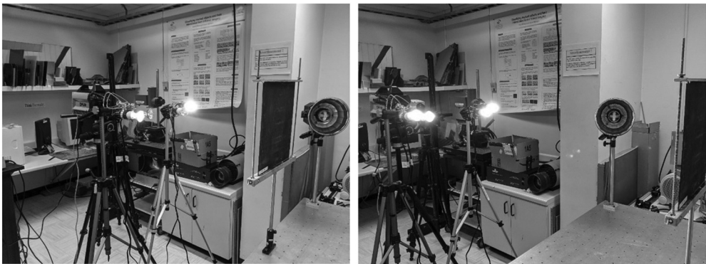
Figure 18. (A) An image of the active thermography experimental setup with two halogen lamps. (B) An image of the active thermography experimental setup with four halogen lamps.
