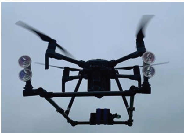
Figure 1. UAV with active thermography capabilities.
