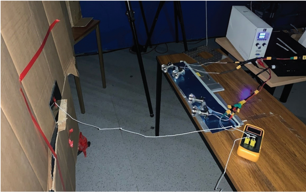
Figure 7. View of the experimental setup of test 6 described in Table 3. The thermocouple probe is bonded to the sample using insulation tape on the cable, the probe is fully exposed.
