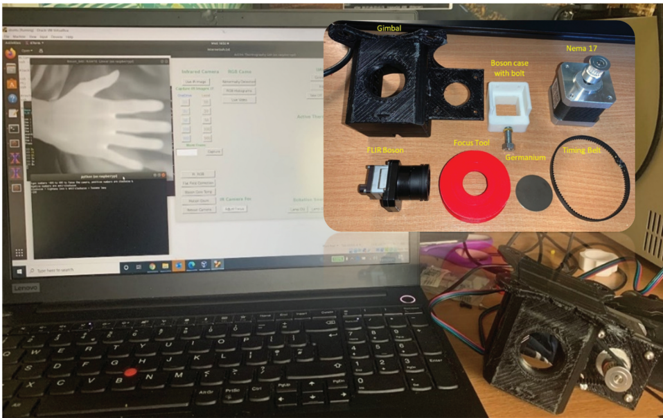
Figure 33. Developed focus mechanism for the FLIR Boson.
