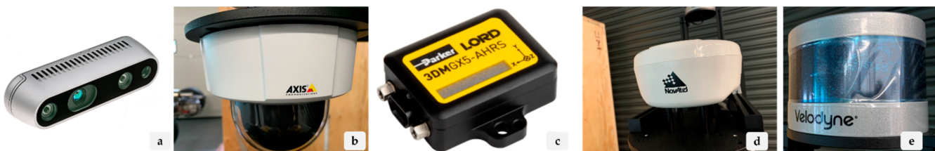
Figure 5. On-board sensors: (a) stereo depth camera; (b) environmental camera; (c) IMU; (d) RTK-GPS; (e) 3D Lidar.
