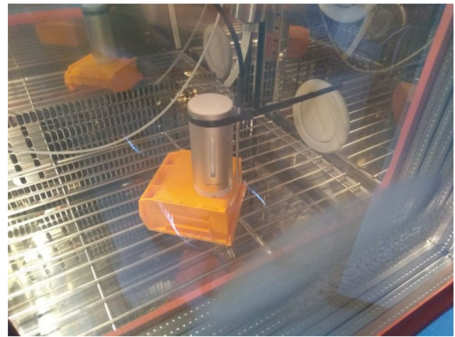
FIGURE 2 A Netatmo temperature sensor in the climate chamber. The thermocouple is attached by a cable tie so that the same parcel of air is measured by both sensors during the test.
