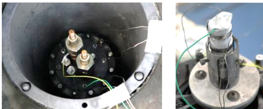
Fig. 2. The EV-ARC chamber (left) and Cell placed in a metallic throne (right).
