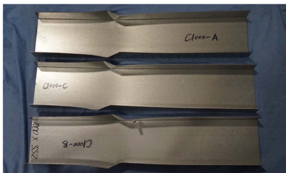
Fig. 13. Failure modes of 1 m long columns with type C cross-section.
