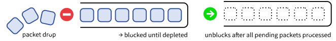
Figure 4: Queue Mitigation: After the packet queue fills up, all incoming packets are dropped until it is empty again.
