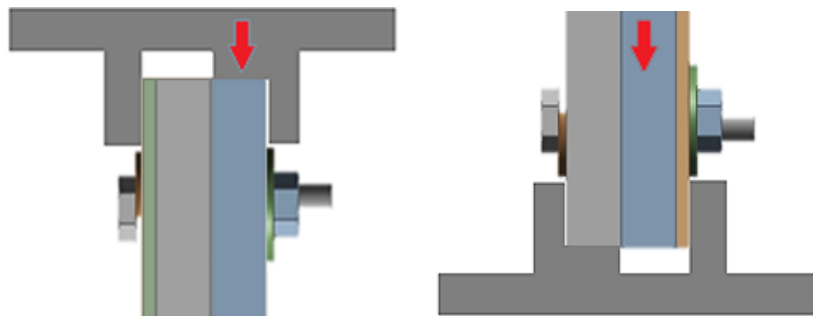
195 Figure 10: Schematic detailed close-up view of specimen, base attached to the supporting block (left); 196 top attached to the load cell block (right).
