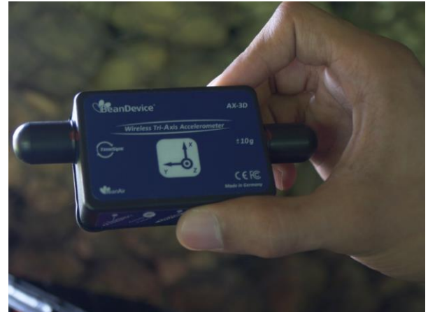
Fig. 6 Bridge instrumentation consisting of 10 wireless triaxial accelerometers
