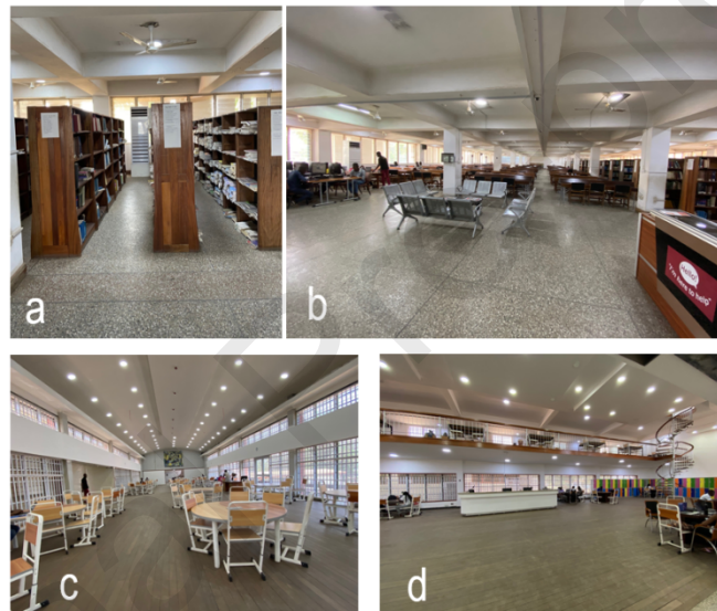
Figure 3—a) new block-west facing windows shaded by the balconies and blocked by the bookshelves, b) new block-second floor with ACs. c) old block-second floor with louvres for natural ventilation and shading, d) old block-ground floor and mezzanine
