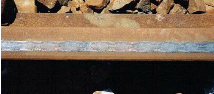
Figure 2.6: Short pitch corrugations (Wilson, 2012)
