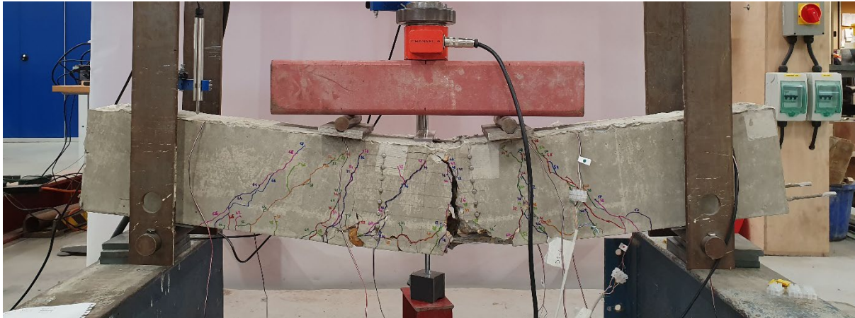
486 Figure 16 Sample B20A-L10 at the end of flexural testing until failure, showing rupture of the bottom 487 reinforcement.
