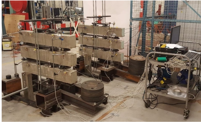
Figure 3. Samples in the sustained loading testing rig
