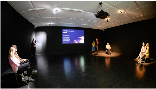
Figure 10. Finalised version of the hertz infrasound installation at The Box at We The Curious, Bristol. Members of the public sit on furniture which has transducers beneath. The subwoofer is located in the far-left corner. Information about hertz is projected onto the wall.
