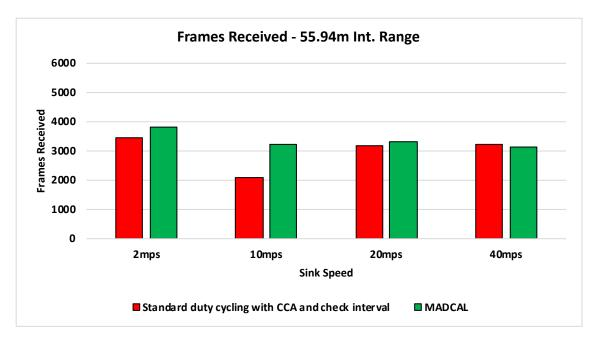
Figure 4.22: Sink Frame Reception, Random Topology. Transmission range 55.94m. MADCAL
