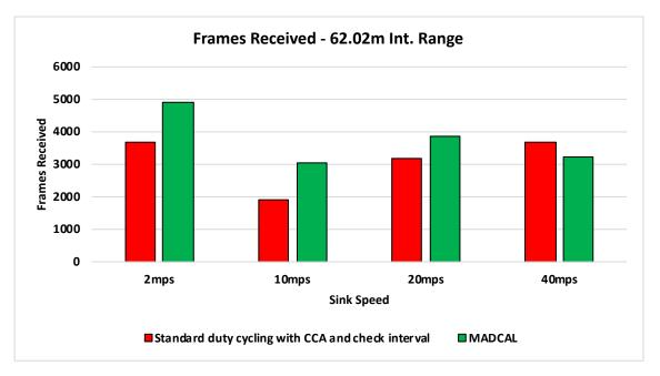
Figure 4.21: Sink Frame Reception, Random Topology. Transmission range 62.02m. MADCAL
