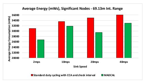
**Figure 4.8:** Average Energy Consumption (mWs), Grid Topology, Significant Nodes. Transmission range 69.13m. MADCAL
