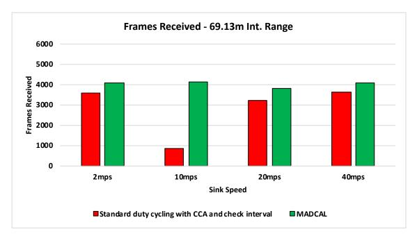
Figure 4.20: Sink Frame Reception, Random Topology. Transmission range 69.13m. MADCAL
