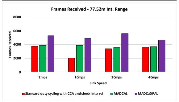
**Figure 5.19:** Sink Frame Reception. Transmission Range 77.52m, Random Topology. MADCaD-PAL
