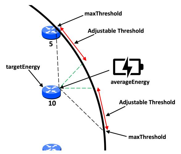
Figure 6.2: Adjustment of threshold based on average and target energy - DMEAAL
