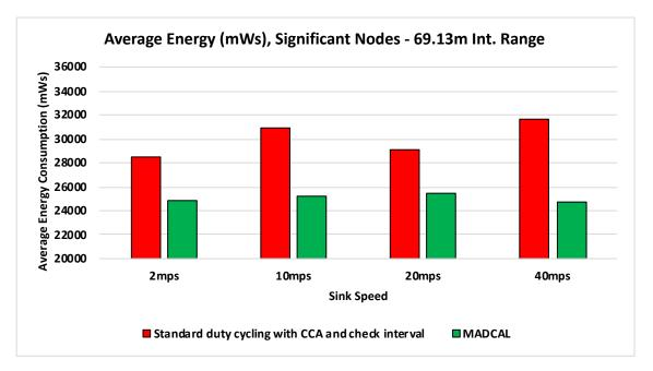
**Figure 4.16:** Average Energy Consumption (mWs), Random Topology, Significant Nodes. Transmission range 69.13m. MADCAL Figure 4.18 is significant in that the transmission range is now strained to a great extent. However, benefits can still be seen with MADCAL in use. As with the grid topology, this is less evident when the sink is moving faster. However, unlike in the equivalent test, shown in Figure 4.10, the benefits in energy consumption are greater overall now.
