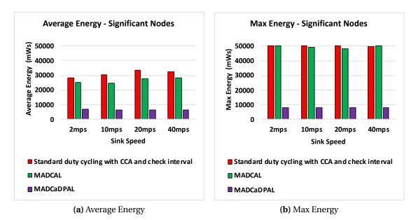
**Figure 5.17:** Average and Maximum Energy Consumption of Significant Nodes (mWs). Transmission Range 62.02m, Random Topology. MADCaDPAL
