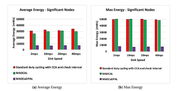
**Figure 5.10:** Average and Maximum Energy Consumption of Significant Nodes (mWs), Grid Topology. Transmission Range 55.94m. MADCaDPAL
