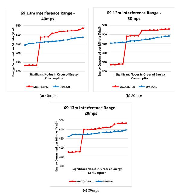
**Figure 6.9:** Balanced Energy Consumption of Significant Nodes (mWs), Grid Topology. Transmission Range 69.13m. DMEAAL
