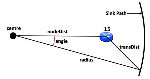
Figure 4.4: Illustration of Calculation of Initial Angle of Threshold - MADCAL
