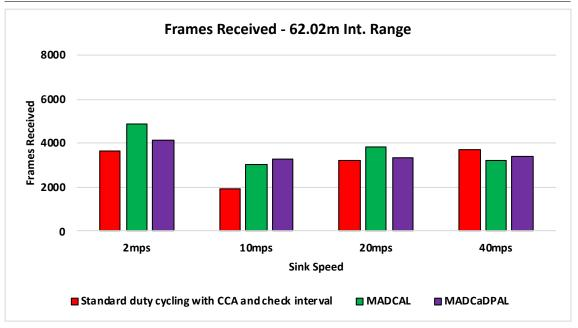
**Figure 5.21:** Sink Frame Reception. Transmission Range 62.02m, Random Topology. MADCaD-PAL
