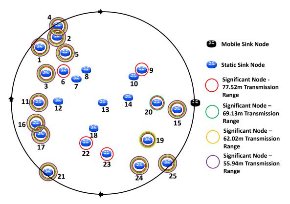
Figure 4.2: Network topology - random with significant nodes.
