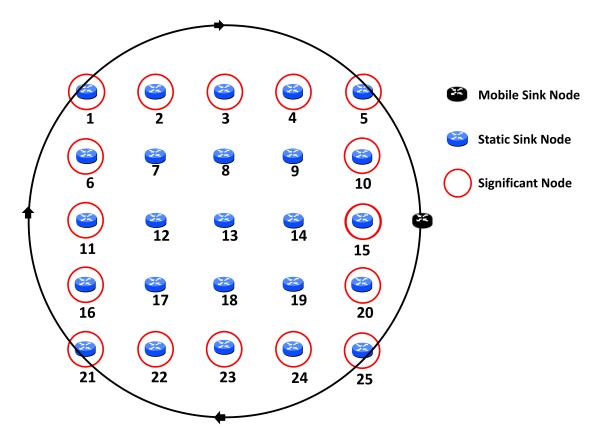
Figure 4.1: Network topology - grid with significant nodes.
