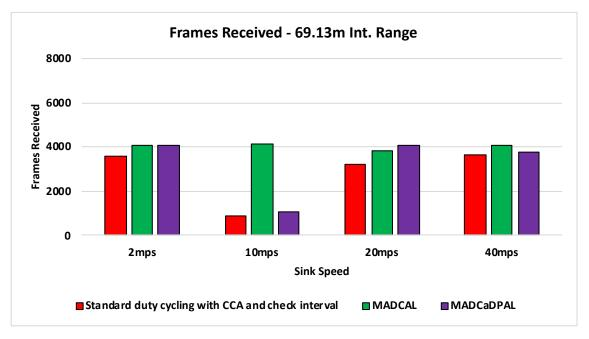
**Figure 5.20:** Sink Frame Reception. Transmission Range 69.13m, Random Topology. MADCaD-PAL
