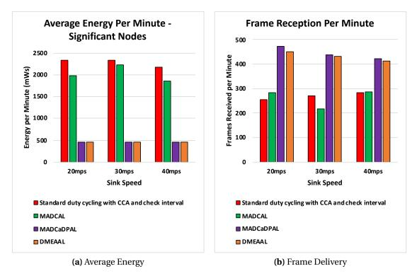
**Figure 6.6:** Average Energy Consumption of Significant Nodes (mWs) and Frame Delivery to Sink, Grid Topology. Transmission Range 62.02m. DMEAAL
