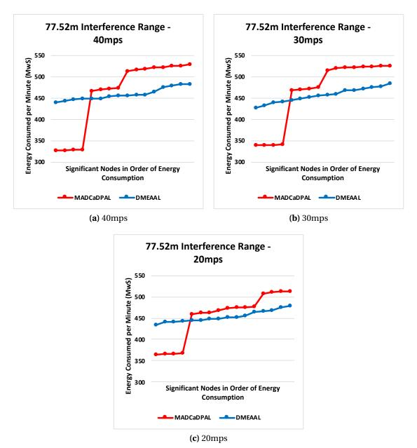
**Figure 6.8:** Balanced Energy Consumption of Significant Nodes (mWs), Grid Topology. Transmission Range 77.52m. DMEAAL
