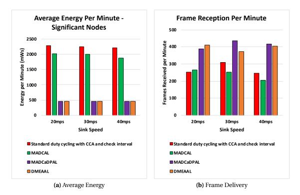
**Figure 6.4:** Average Energy Consumption of Significant Nodes (mWs) and Frame Delivery to Sink, Grid Topology. Transmission Range 77.52m. DMEAAL
