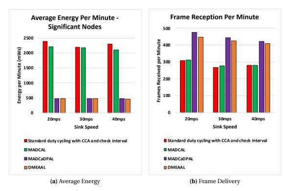
**Figure 6.5:** Average Energy Consumption of Significant Nodes (mWs) and Frame Delivery to Sink, Grid Topology. Transmission Range 69.13m. DMEAAL
