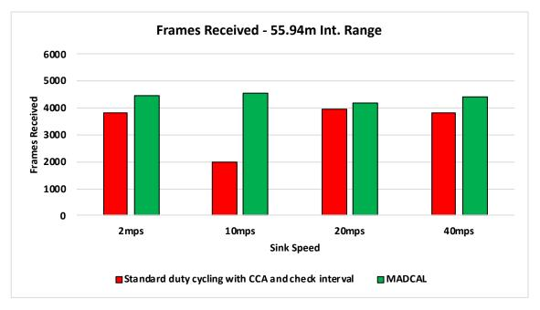
Figure 4.14: Sink Frame Reception, Grid Topology. Transmission range 55.94m. MADCAL
