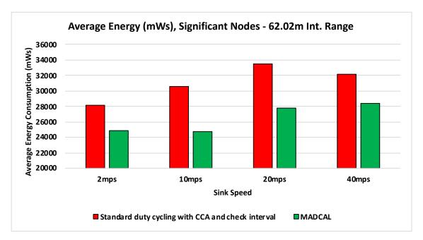
**Figure 4.17:** Average Energy Consumption (mWs), Random Topology, Significant Nodes. Transmission range 62.02m. MADCAL
