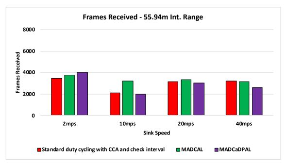
**Figure 5.22:** Sink Frame Reception. Transmission Range 55.94m, Random Topology. MADCaD-PAL
