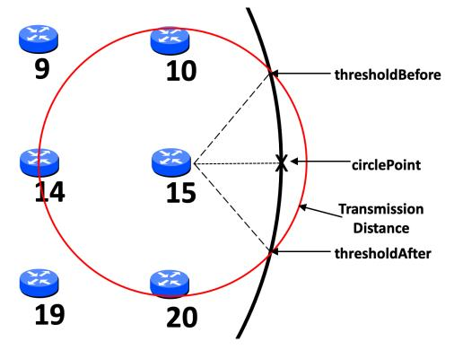
Figure 4.5: Illustration of Initial Threshold Calculation - MADCAL
