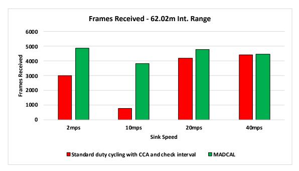
Figure 4.13: Sink Frame Reception, Grid Topology. Transmission range 62.02m. MADCAL
