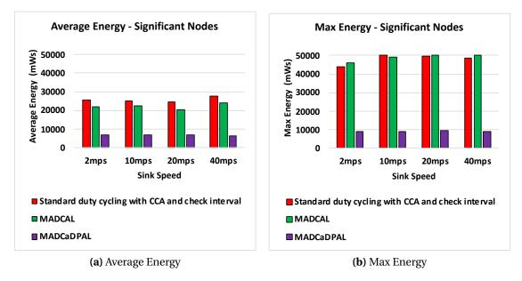
**Figure 5.15:** Average and Maximum Energy Consumption of Significant Nodes (mWs). Transmission Range 77.52m, Random Topology. MADCaDPAL
