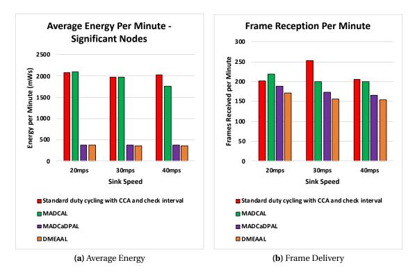
**Figure 6.15:** Average Energy Consumption of Significant Nodes (mWs) and Frame Delivery to Sink. Transmission Range 55.94m. DMEAAL
