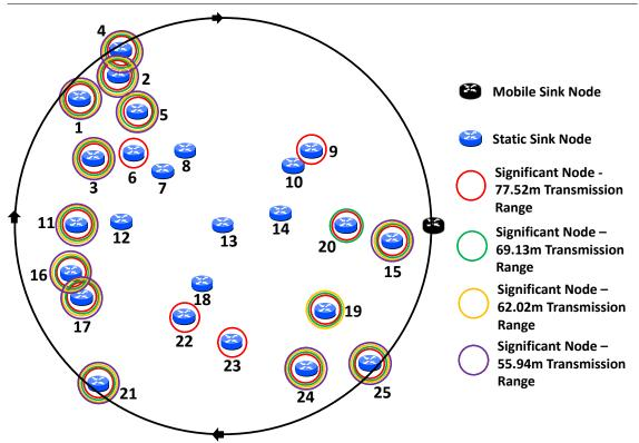
Figure 5.4: Network topology - random with significant nodes.
