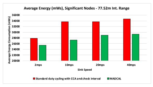
**Figure 4.7:** Average Energy Consumption (mWs), Grid Topology, Significant Nodes. Transmission range 77.52m. MADCAL
