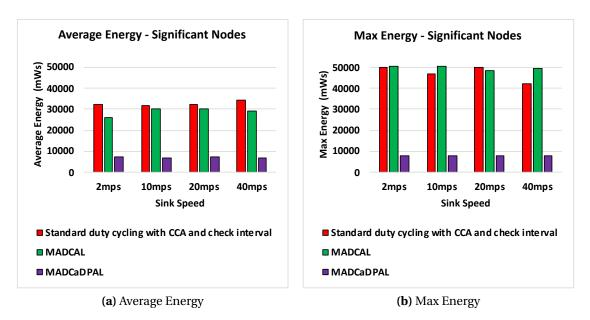
**Figure 5.9:** Average and Maximum Energy Consumption of Significant Nodes (mWs), Grid Topology. Transmission Range 62.02m. MADCaDPAL
