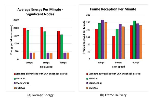
**Figure 6.13:** Average Energy Consumption of Significant Nodes (mWs) and Frame Delivery to Sink, Random Topology. Transmission Range 69.13m. DMEAAL
