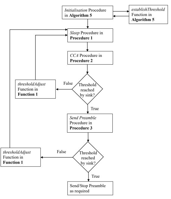
Figure 6.3: DMEAAL Control Flow
