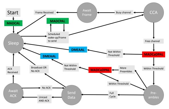
Figure 6.1: Lightweight CSMA/CA MAC Implementation with DMEAAL
