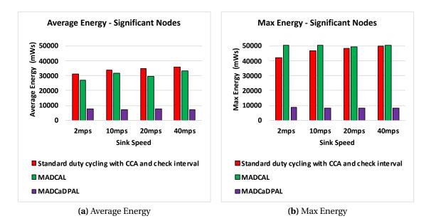
**Figure 5.8:** Average and Maximum Energy Consumption of Significant Nodes (mWs), Grid Topology. Transmission Range 69.13m. MADCaDPAL
