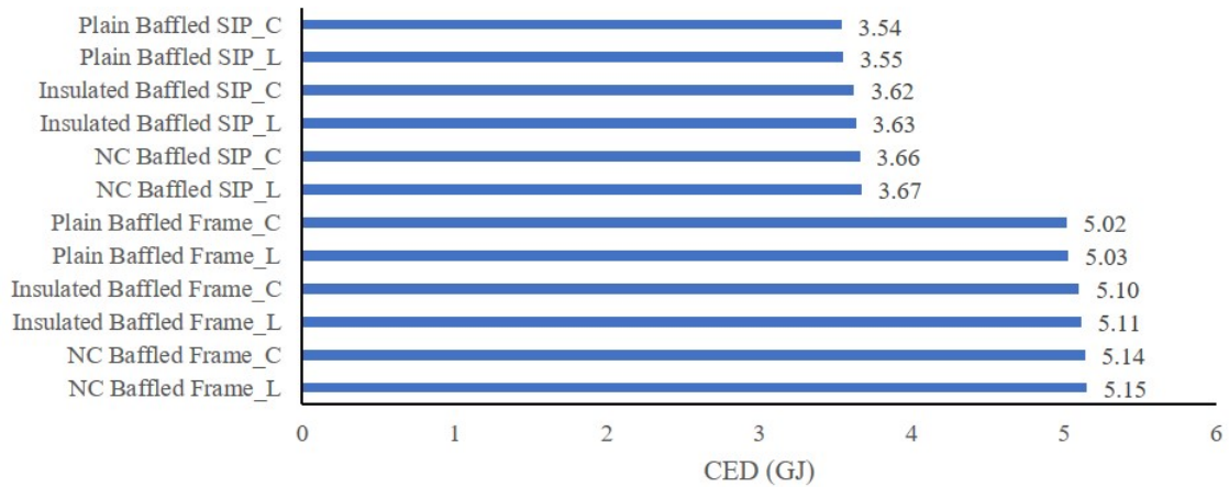
Figure 5.2: CED impact comparison for baffled configuration scenarios. NC – night cover, L – linear, C – circular
