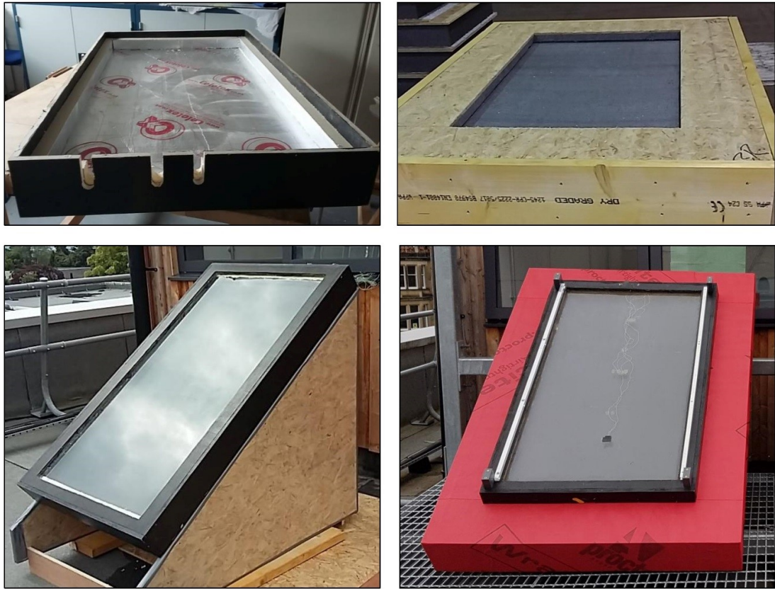
Figure 3.13: Pictures of the empty frame (top-left) and empty SIP (top-right), showing the different extent of insulation. The ICS collector in-situ is shown in the frame (bottom-left) and the SIP (bottom-right)
