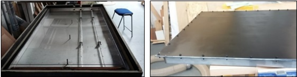
Figure 3.7: Configuration and placement of the internal baffle plate, with the supporting pillars, and the storage tank and absorber plate bolted together
