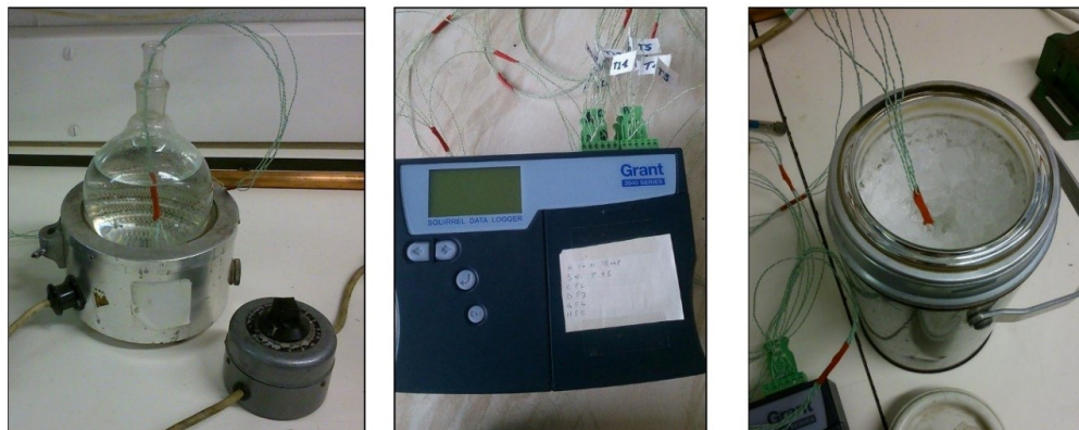
Figure 3.9: Boil and ice test apparatus. From left to right: hot water bath; Grant SQ2040 data logger; thermos flask
