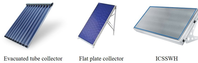
Figure 1.2: The main types of solar water heaters. The evacuated tube and flat plate collectors require an external water storage tank while this is integrated in the ICSSWH variant
