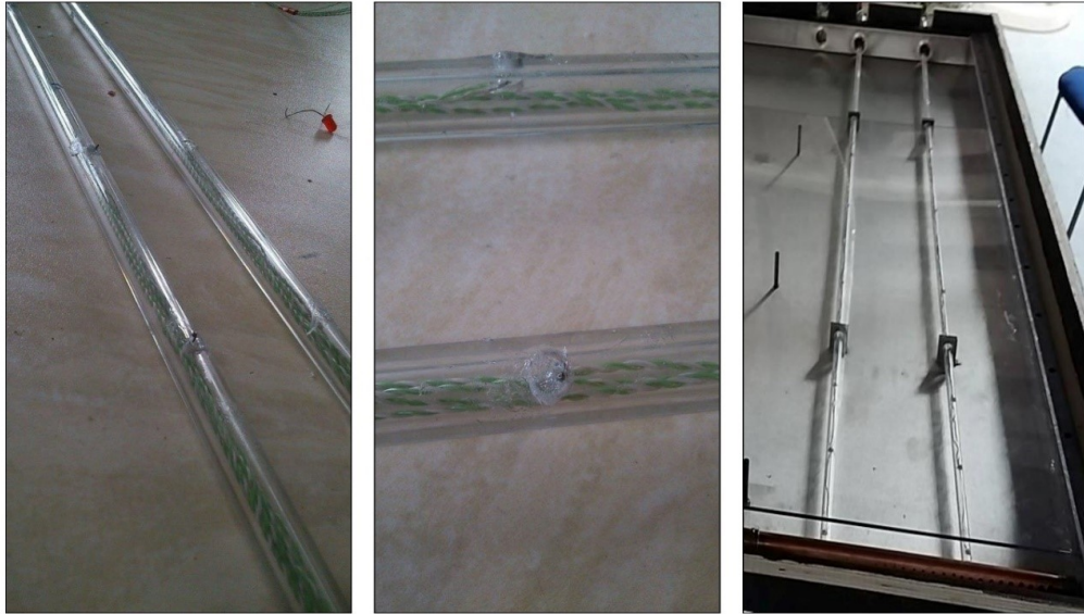
Figure 3.11: Thermocouples inserted into polycarbonate tubing to keep them stable within the water body. The photo on the right shows the thermocouple placement inside the baffled tank, the rods supported with small plastic supports
