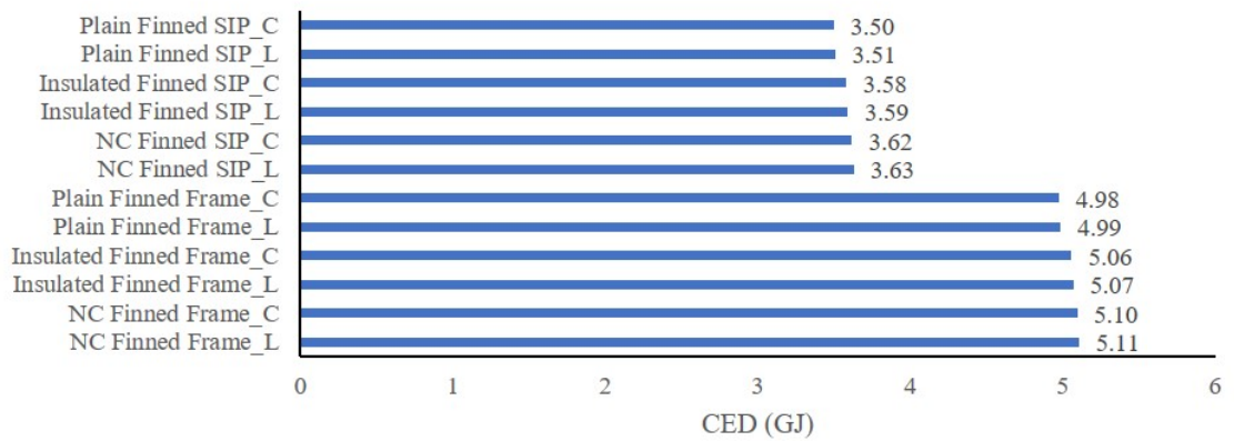
Figure 5.4: CED impact comparison for finned configuration scenarios. NC – night cover, L – linear, C - circular
