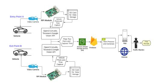
Figure 12. Flowchart of IoT-enabled Speed Monitoring System.
