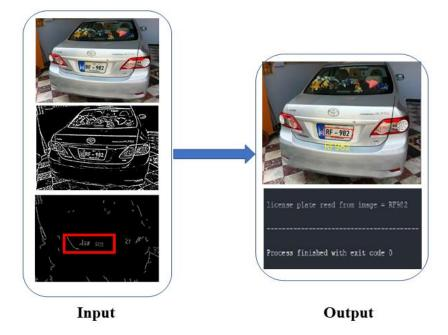
Figure 1. License plate detection and character segmentation.
