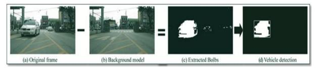
Figure 2. Background subtraction to remove negative points.
