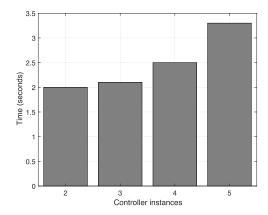
Fig. 11. DDoS attack remediation latency.
