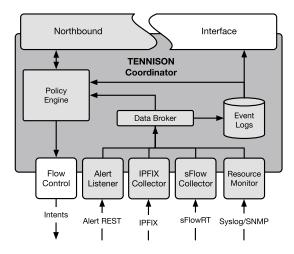
Fig. 2. TENNISON coordinator subsystems and SBI.
