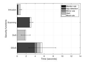
Fig. 9. Attack remediation latency - single controller.
