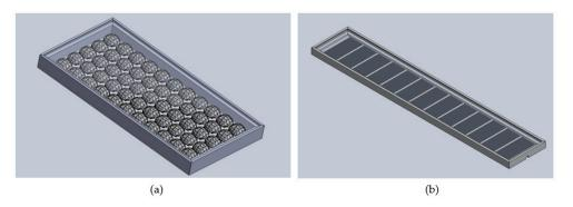
**Figure 2.** Visual representation of the (a) GOCRSH\_A module and (b) the flat PV module (representation is not to scale).
