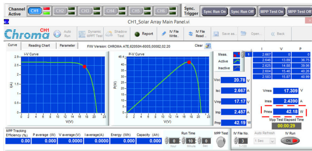
FIGURE 27. I-V and P-V curves under uniform conditions at an irradiance of 700 W/m 2 .
