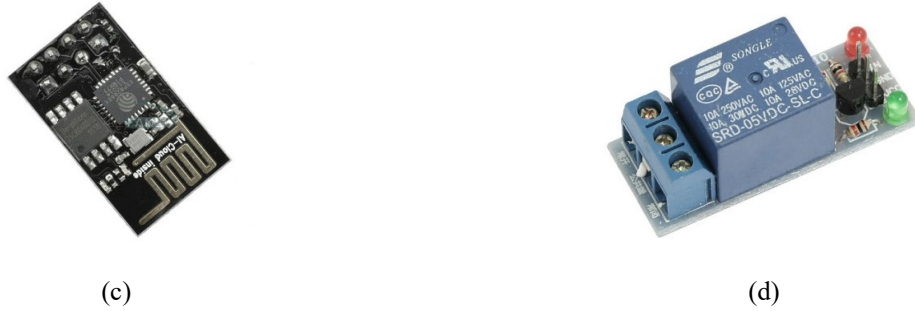
Fig. 5 - (a) Current sensor (ACS712); (b) Voltage sensor (ZMPT101b); (c) WiFi chip (ESP8266); (d) switching relay
