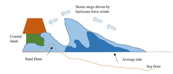
Figure 2.1 Schematic diagram of storm surge rising above mean sea level
