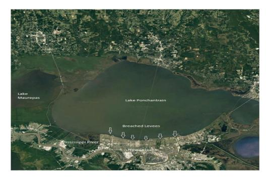
Figure 5.9 Storm surge from the Lake Pontchartrain breaching the levee in the City of New Orleans [Image source: Google Earth]
