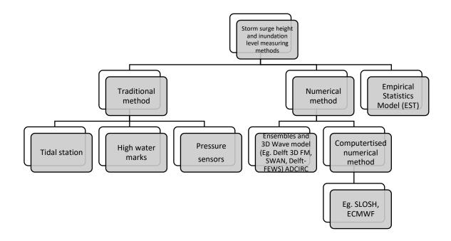
Figure 3.9 Illustration of storm surge measuring methods
