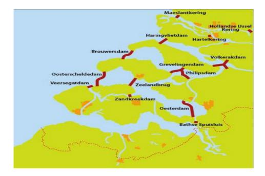
Figure 2.17. The Delta region of the Netherlands protected by various coastal barriers (storm surge barriers, sluices, dams) [source: Deltawerken Online (2004)]
