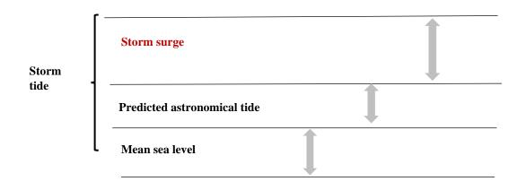
Figure 2.2 Difference between storm surge, storm tide, high tide and MSL
