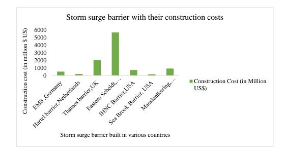
Figure 2.19 Global storm surge barriers and their corresponding construction costs [source: Linham & Nicholls (2010)]
