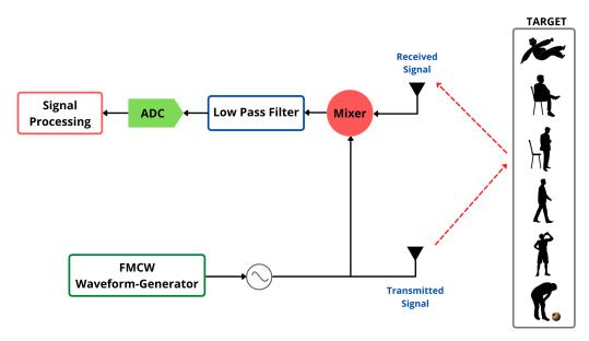
Figure 3. Block diagram of the FMCW RADAR scheme for distinct activity recognition.
