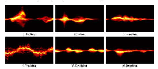
Figure 5. Samples of the acquired micro-Doppler signatures of six different activities.
