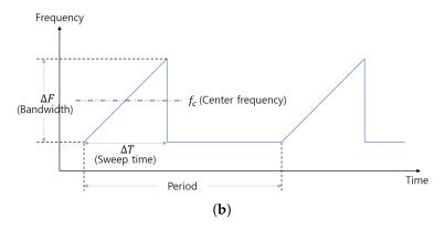
Figure 2. FMCW RADAR (a) structure (b) signal produced from the waveform-generator [50].
