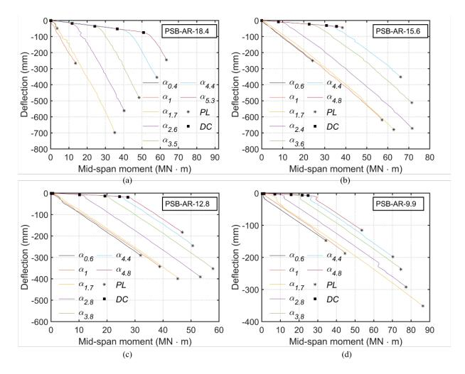
Fig. 3. Mid-span moment versus deflection.
