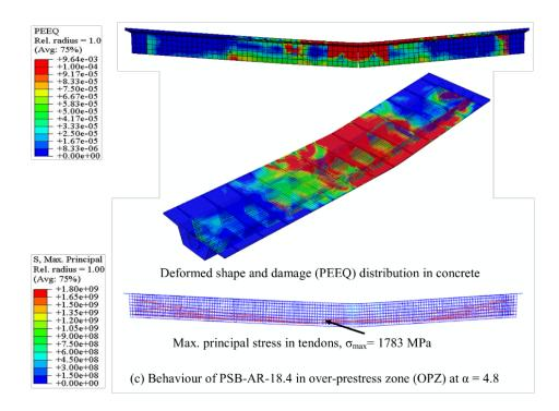
Fig. 10. Failure modes at PDZ ( $\alpha$ =1.0), NPZ ( $\alpha$ =2.6), OPZ ( $\alpha$ =4.8) for models with the same aspect ratio but different normalized prestress factor ( $\alpha$ ) (cont'd).
