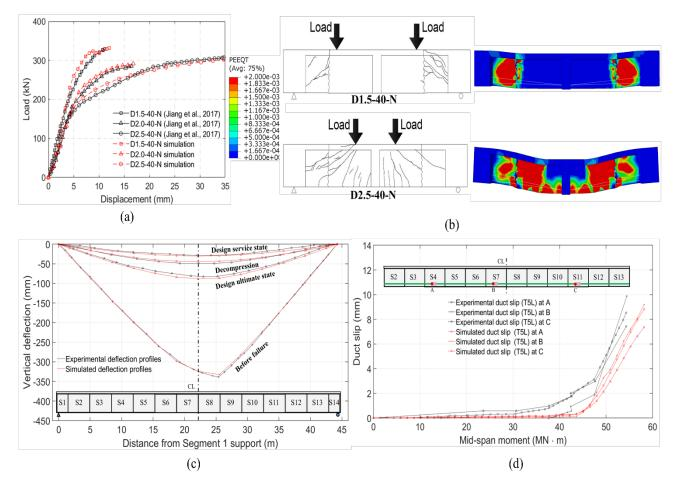
**Fig 2.** (a) Comparison of the simulated and experimental (a) load-deflection curves and (b) crack patterns by Jiang *et al.* [41]; (b) comparison of the simulated and experimental (c) deflection profile and (d) duct slips of T5L at different loading stages by Takebayashi *et al.* [28].
