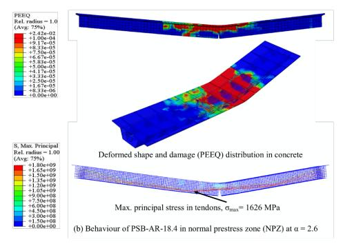
**Fig. 10.** Failure modes at PDZ ( $\alpha$ =1.0), NPZ ( $\alpha$ =2.6), OPZ ( $\alpha$ =4.8) for models with the same aspect ratio but different normalized prestress factor ( $\alpha$ ).
