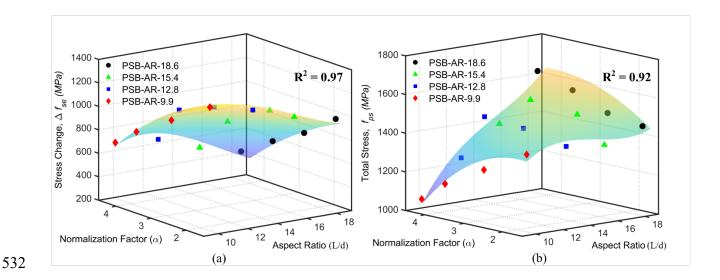
Fig. 12. Response surface showing the relationship between normalized prestress factor  $\alpha$  and aspect ratio L/d w.r.t. (a) stress change  $\Delta f_{se}$  and (b) total stress  $f_{ps}$ .
