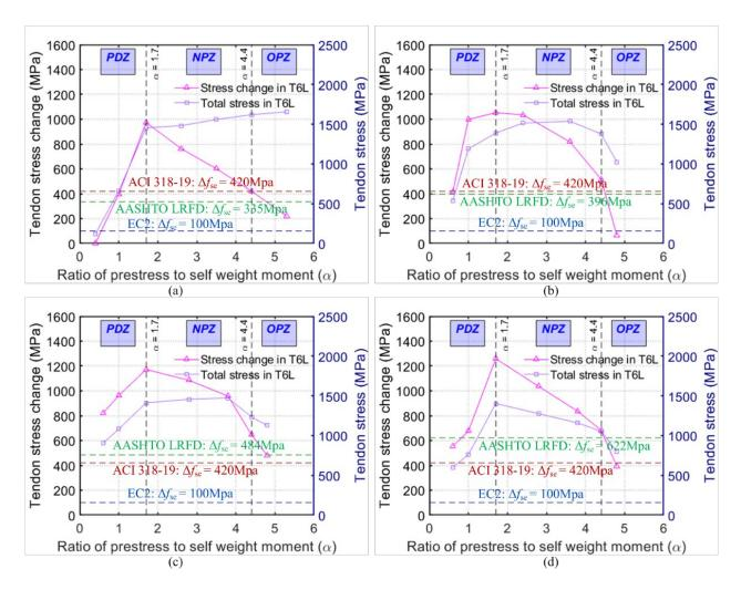
**Fig. 8.** Effects of the variations in effective prestress on stress changes and the maximum tension stress at BF with different aspect ratio (a) PSB-AR-18.4, (b) PSB-AR-15.6, (c) PSB-AR-12.8, and (d) PSB-AR-9.9.
