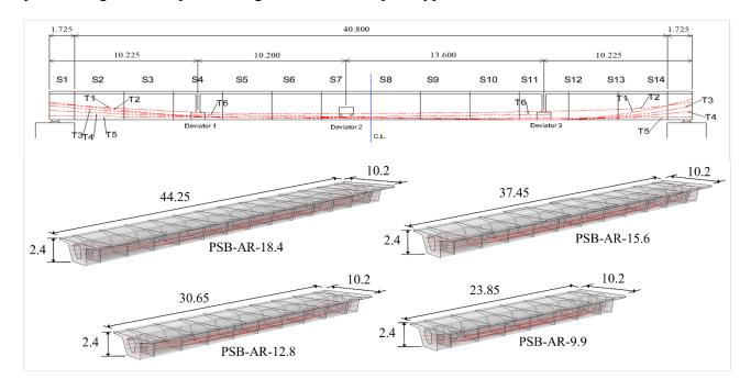
**Fig 1.** Schematic diagram with tendon profile of prototype PCSB (the non-prestressing reinforcement is not shown) [28] and geometric details of numerical models (dimensions in m).
