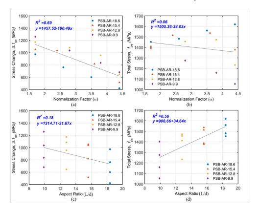
Fig. 11. Influence of the normalized prestress factor  $\alpha$  and aspect ratio L/d on stress change  $\Delta f_{se}$  and total stress  $f_{ps}$ .
