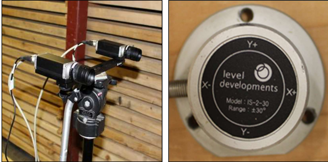
Fig. 1: Image of the stereo camera system (left) and inclinometer (right).
