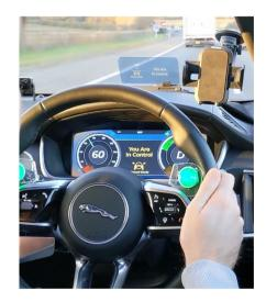
**Fig.8** The left-hand image shows the green buttons on the steering wheel and the infotainment display (ambient blue lighting indicates that the vehicle is in automated mode). The driver-facing camera can
