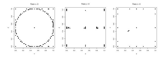
Figure 5: Superimposition of scaled hole feature coordinates for all the data on the specified face of the cube.
