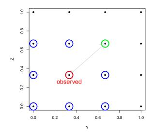
Figure 14: Illustration of hill-climbing search to nearest predictive mode. The [0, 1] interval is divided into a N by N grid, in this case N = 4. The kernel density is estimated at the discrete black points. A feature is observed at a specific position, shown in red, and the mode is located by moving in increasing steps between neighboring grid positions.
