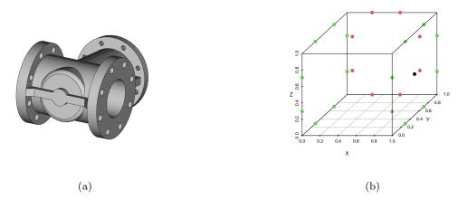
Figure 4: Example of a valve body from CAD design database. Figure 4a shows an image of a valve design and Fig. 4b the scaled positions of the extracted hole features. The different colors are used to identify the different diameters of the holes
