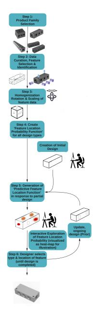
Figure 3: System schematic for feature prediction through Bayesian updating.
