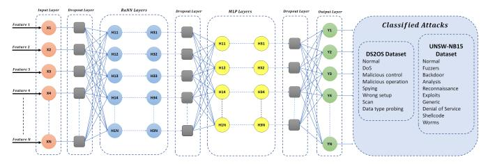
FIGURE 1. Proposed HDRaNN attack detection model.
