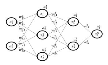
Figure 2: Structural diagram of a three-layer fully connected neural network
