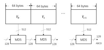
Figure 5: Lightweight encryption method for MD5 group processing
