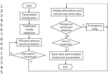
Figure 4: Stop mechanism flowchart
