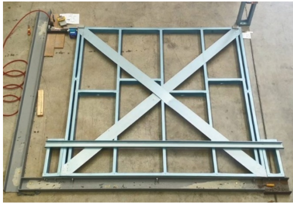
Fig. 16. Tested frame with 150 mm strap bracing [72]
