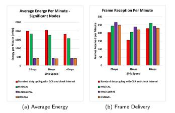
**Figure 18:** Average Energy Consumption of Significant Nodes (mWs) and Frame Delivery to Sink. Interference Range 69.13m
