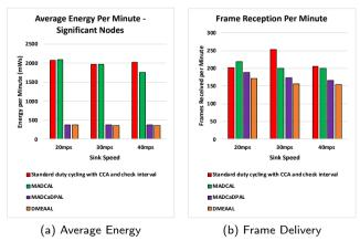
**Figure 20:** Average Energy Consumption of Significant Nodes (mWs) and Frame Delivery to Sink. Interference Range 55.94
