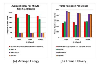
**Figure 11:** Average Energy Consumption of Significant Nodes (mWs) and Frame Delivery to Sink. Interference Range 62.02m
