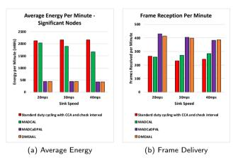
**Figure 12:** Average Energy Consumption of Significant Nodes (mWs) and Frame Delivery to Sink. Interference Range 55.94m
