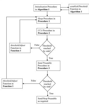
Figure 8: DMEAAL Control Flow
