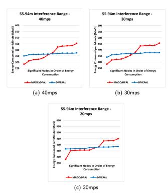
**Figure 24:** Balanced Energy Consumption of Significant Nodes (mWs). Interference Range 55.94m
