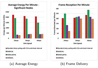
**Figure 19:** Average Energy Consumption of Significant Nodes (mWs) and Frame Delivery to Sink. Interference Range 62.02m
