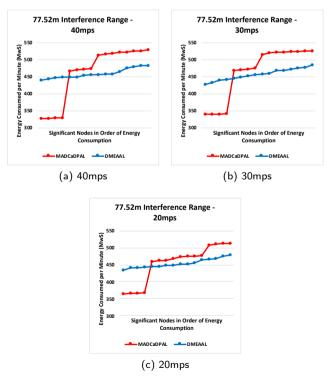
**Figure 13:** Balanced Energy Consumption of Significant Nodes (mWs). Interference Range 77.52*m*
