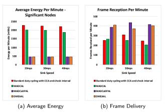
**Figure 9:** Average Energy Consumption of Significant Nodes (mWs) and Frame Delivery to Sink. Interference Range 77.52m
