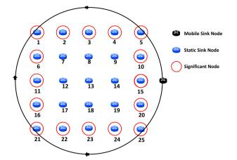
Figure 3: Network topology - grid with significant nodes.
