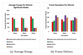
**Figure 17:** Average Energy Consumption of Significant Nodes (mWs) and Frame Delivery to Sink. Interference Range 77.52m
