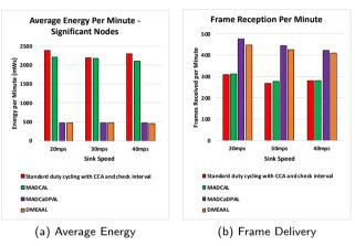
**Figure 10:** Average Energy Consumption of Significant Nodes (mWs) and Frame Delivery to Sink. Interference Range 69.13m
