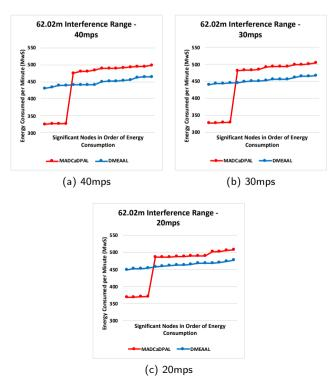
**Figure 15:** Balanced Energy Consumption of Significant Nodes (mWs). Interference Range 62.02m
