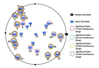
Figure 4: Network topology - random with significant nodes.
