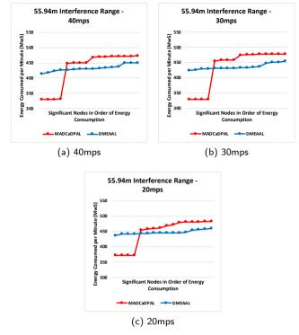
**Figure 16:** Balanced Energy Consumption of Significant Nodes (mWs). Interference Range 55.94m
