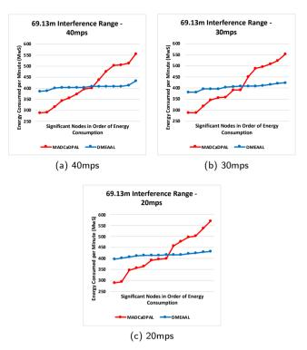
**Figure 22:** Balanced Energy Consumption of Significant Nodes (mWs). Interference Range 69.13*m*
