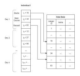
Figure 1. Example of solution encoding.
