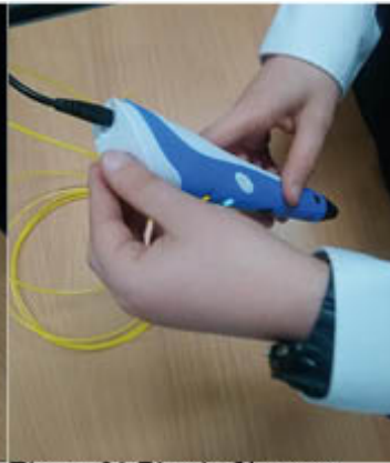
Figure 31 Plastic filament being loaded into 3D printing pen
