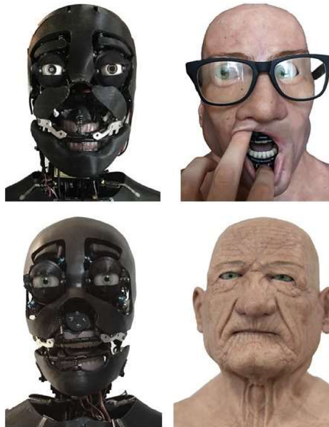
Figure 3. Realistic humanoid robots (RHRs) with EAI ‘Euclid’ and ‘Baudi’ implemented in the human–robot interaction (HRI) experiment.
