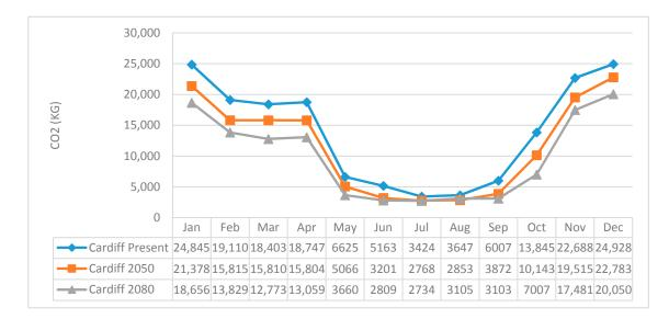
Figure 9. CO<sub>2</sub> production in the current, 2050, and 2080 time slices.
