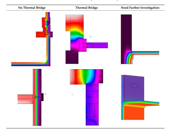
**Table 2.** Thermal bridge analysis with Therm and Psi Therm. From top to bottom: left column curtain walls; middle column: wall-to-door and louver; and right column: Parapet 2D and 3D.
