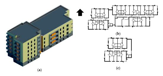
**Figure 4.** 3D model (**a**); (**b**) ground floor to 3rd floor; and (**c**) 4th and 5th floor, the arrow shows the north side.
