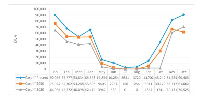
Figure 7. Heating loads in the current, 2050, and 2080 time frames.
