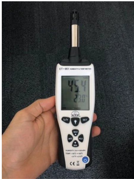
Fig. 6. Thermo-hygrometer for indoor air temperature recordings
