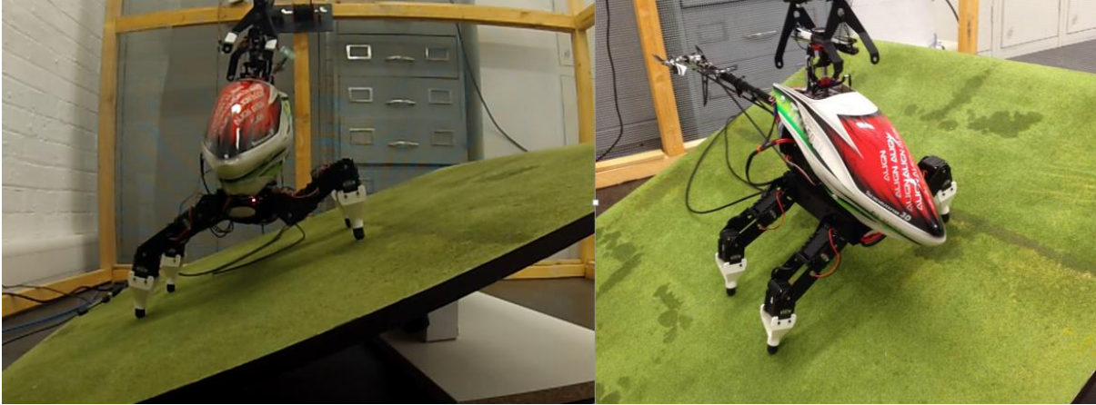
Figure 6-9 Robotic landing gear during slope landing
