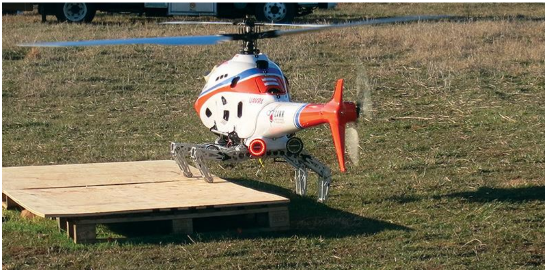
Figure 2-4 Georgia Tech robotic landing gear on Robot Buzz 2 helicopter during test flight [15]
