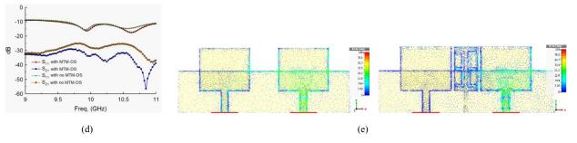
Fig.13. Antenna array (a) before apply MTM isolator shield and (b) after apply MTM isolator shield, (c) circuit of two patches with MTM-DS, (d) Sparameter responses, (e) surface current densities at 10.65 GHz [117].
