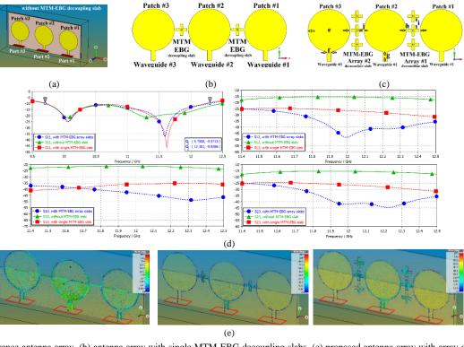
Fig.6. (a) Reference antenna array, (b) antenna array with single MTM-EBG decoupling slabs, (c) proposed antenna array with array of MTM-EBG decoupling slabs, (d) S-parameters performances, (e) distributed surface currents at resonance frequency of 10 GHz [110].
