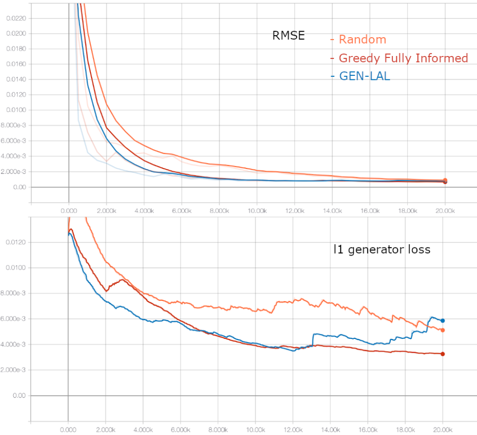
Figure 5. Plots of RMSE corresponding to Figure 4 on the test set and L1 parameter loss-convergence behaviors for the random, greedy fully Informed and GEN-LAL adaptive-learning sampling methods. Top: RSME; bottom: L1 generator loss (also translucent in above plot).
