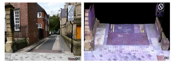
**Fig. 4.** Field site: The field site was located adjacent to St James Church on Northumberland Road, Newcastle Upon Tyne, UK Grid Reference NZ 25112 64814. (a) Conventional photograph of the field site. (b) Point cloud panorama of the site captured using the Faro Focus 3D X Series phased-based laser scanner. The three surfacing materials studied are (i) surface dressing, (ii) dense bitumen macadam, and (iii) hot rolled asphalt.
