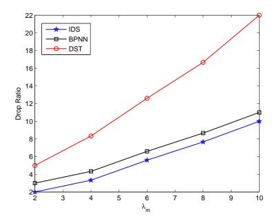
Fig. 7: Drop ratio under different values of malicious nodes arrival rates
