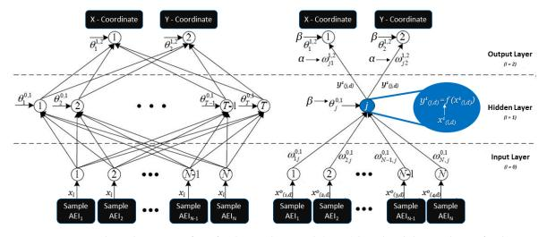
**Figure 2.** Topological mapping of Artificial Neural Network (ANN)-based mobility prediction for the London Underground and Overground (LUO) environment.
