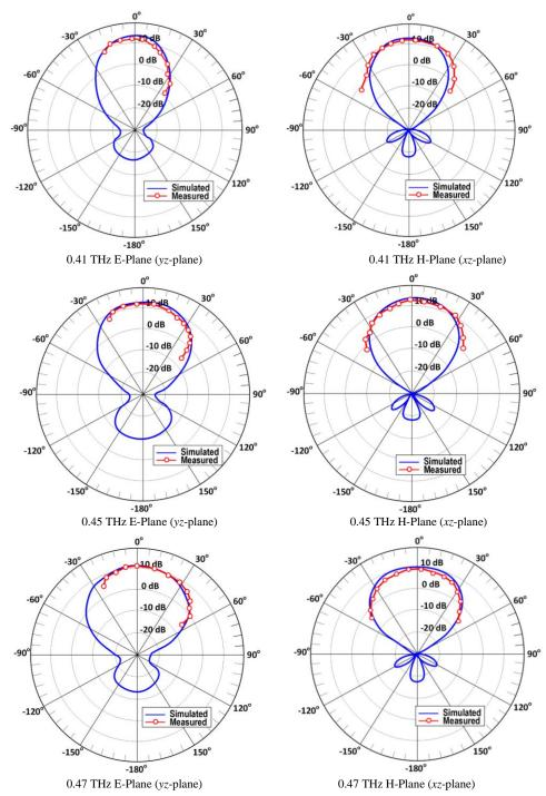
Fig.5. Simulated and measured E- and H-planes radiation patterns of the proposed on-chip antenna modelled by an array of  $11\times11$  circular patches at 0.41 THz, 0.45 THz and 0.47 THz.
