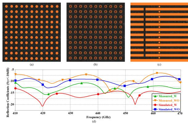
Fig.2. Fabricated prototypes of the reference, i.e. without (WO) metasurface slots, and the proposed, i.e. with (W) metasurface slots, on-chip antennas. (a) Topview of the reference on-chip antenna, (b) top-view of the proposed on-chip antenna, (c) back-view of both op-chip antennas, and (d) the simulated and measured reflection-coefficient response.
