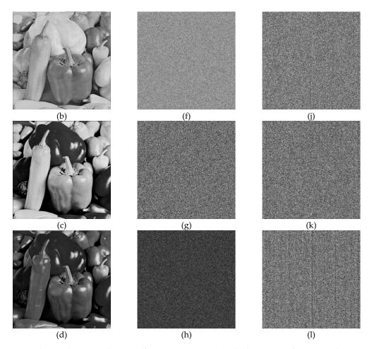
Figure 9. Plain and encrypted images of pepper ( $512 \times 512$ ); (a–d) Plain image of pepper and respected three channels of a pepper test image. (e–h) Shuffled image of pepper and respected three channels of pepper image. (i–l) Encrypted image of pepper and respected three channels of pepper test image using Julia fractals.
