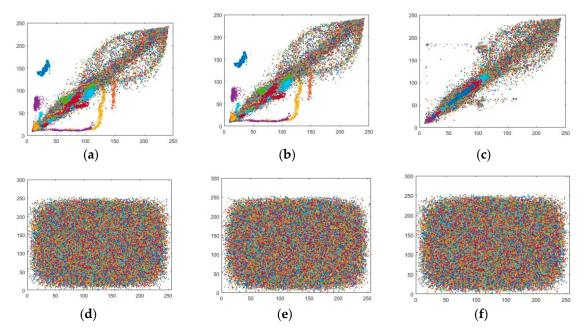
**Figure 17.** Correlation coefficient of splash image ( $512 \times 512$ ); (**a–c**) Correlation coefficient of plain splash image for three directions of a = Horizontal (H-D), b = Diagonal (D-D) and, c = Vertical (V-D). (**d–f**) Correlation coefficient of encrypted splash image for three directions of d = Horizontal (H-D), e = Diagonal (D-D) and f = Diagonal (V-D).
