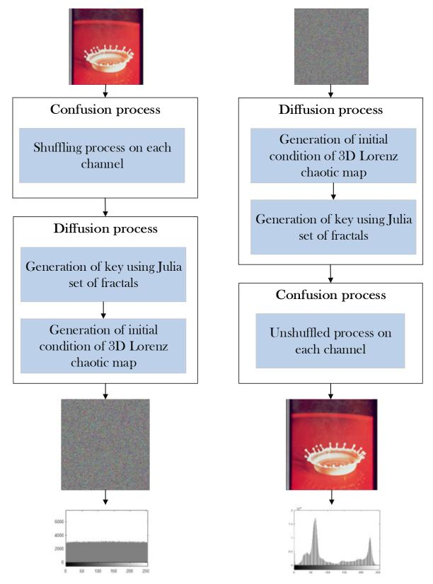
Figure 4. Encryption and decryption process.
