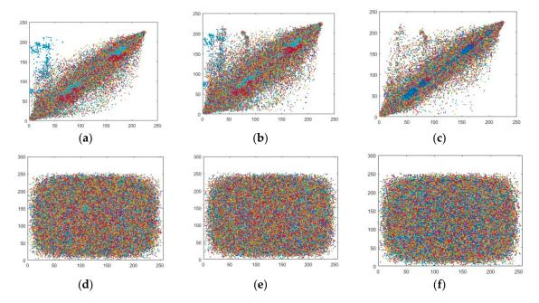
**Figure 18.** Correlation coefficient of pepper image (512  $\times$  512); (**a**–**c**) The correlation coefficient of plain pepper image for three directions of a = Horizontal (H-D), b = Diagonal (D-D) and, c = Vertical (V-D). (**d**–**f**) The correlation coefficient of encrypted pepper image for three directions of d = Horizontal (H-D), e = Diagonal (D-D) and f = Vertical (V-D).
