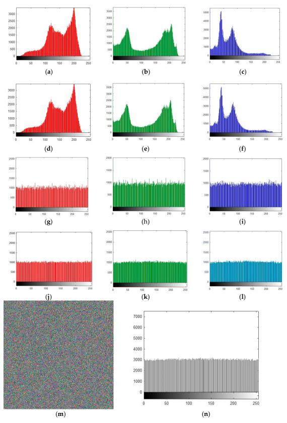
**Figure 16.** Plain and encrypted histogram of pepper image ( $512 \times 512$ ); (a–c) Plain histograms for three grey channels of pepper image. (d–f) Shuffled histograms for three grey channels of pepper image. (g–i) Encrypted three channels of pepper image using Julia fractals. (j–l) Final histograms of three channels using 3D Lorenz chaotic maps. (m,n) Final histogram of combined three channels for the pepper test image.
