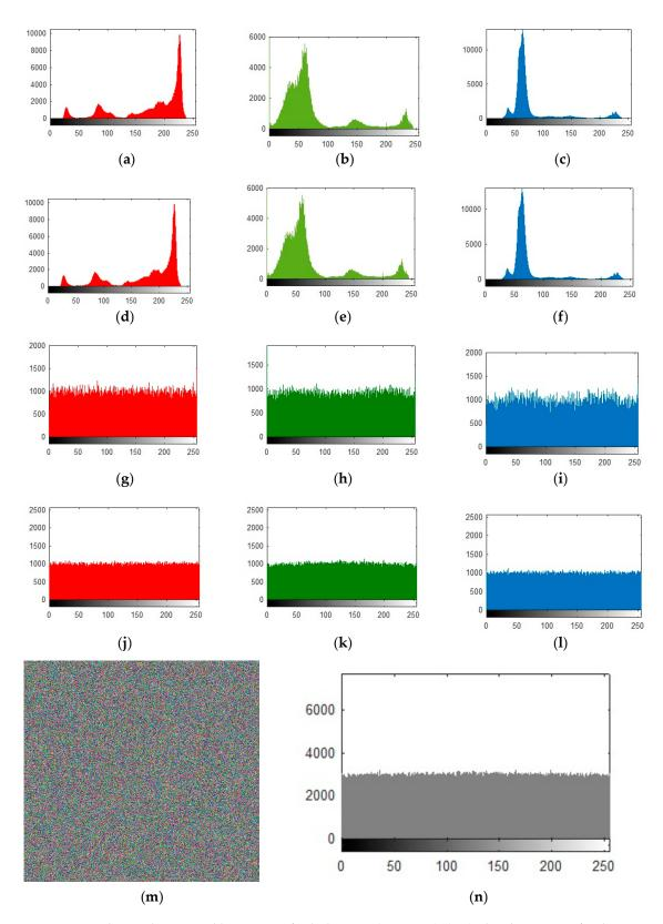
Figure 15. Plain and encrypted histogram of splash image ( $512 \times 512$ ); (a-c) Plain histograms for three grey channels of splash image. (d-f) Shuffled histograms for three grey channels of splash image. (g-i) Encrypted three channels of splash image using Julia fractals. (j-l) Final histograms of three channels using 3D Lorenz chaotic maps. (m,n) Final histogram of combined three channels for the splash test image.
