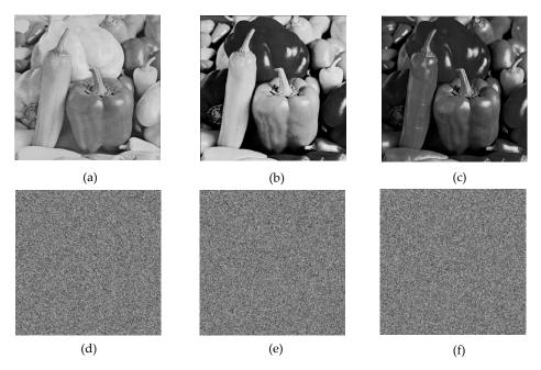
**Figure 10.** Plain and encrypted images of pepper  $(512 \times 512)$ ; (a–c) Three respected plain channels of a pepper test image. (d–f) The final encrypted channels using 3D Lorenz chaotic maps.
