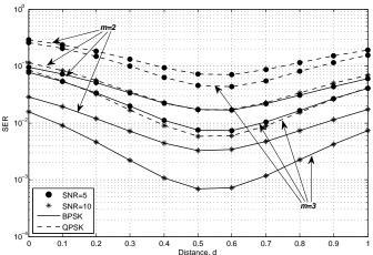
FIGURE 5. Performance comparison of STANC schemes in terms of SER Vs Relay Distance over Nakagami fading channels.
