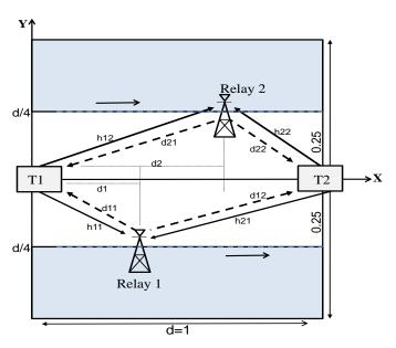
FIGURE 1. STANC System Model under path loss effect.
