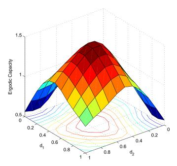
FIGURE 9. Ergodic capacity Vs Relay positioning over Nakagami-m=2 fading channels with L=2 and SNR=10
