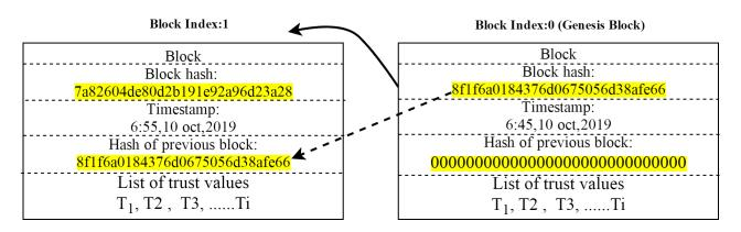
FIGURE 6. Structure of block in blockchain.
