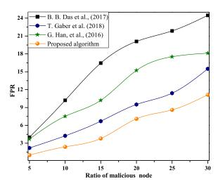
FIGURE 9. Impact of ratio of malicious beacon node on FPR.
