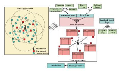
FIGURE 3. Blockchain-based trust management model.
