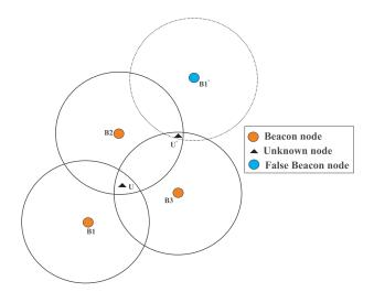
FIGURE 1. Sensor localization example in hostile environments.
