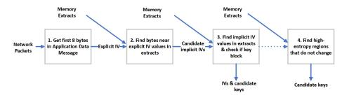
Figure 6-4: TLS Extension GCM Memory Analysis Flow
