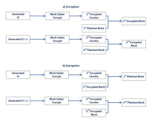
Figure 2-2: CTR Encryption and Decryption Process
