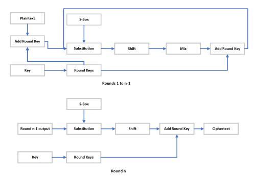
Figure 2-3: AES Encryption Process
