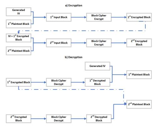
Figure 2-1: CBC Mode Encryption and Decryption Process
