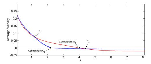
Fig. 9. Dynamic responses of the capsule systems with the EM (blue dotted) and the LM (red dotted) constructed under variation of the mass ratio  $\lambda$ , obtained for h = 1.8,  $\omega = 1.0$ ,  $\rho = 4.0$  and v = 1.2.
