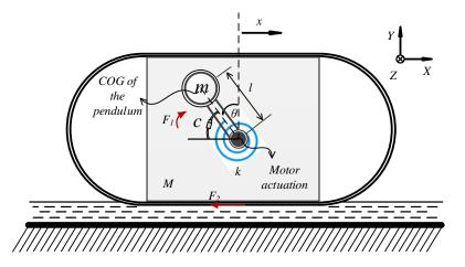
Fig.1. Schematic of the vibro-driven underactuated encapsulated system.
