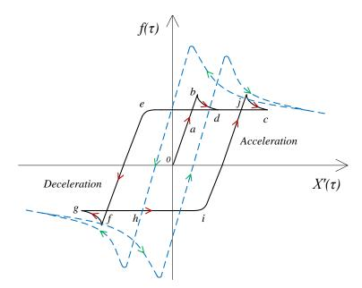
**Fig.3.** Schematic of the reversible (black solid line) and non-reversible (blue dashed line) characteristics of the friction forces.
