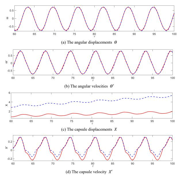
Fig. 5. Friction-induced vibrational response of the system with the EM (blue dashed lines) and system with the LM (red solid lines), obtained for  $\lambda = 2.5$ ,  $\rho = 2.0$  and v = 1.0.
