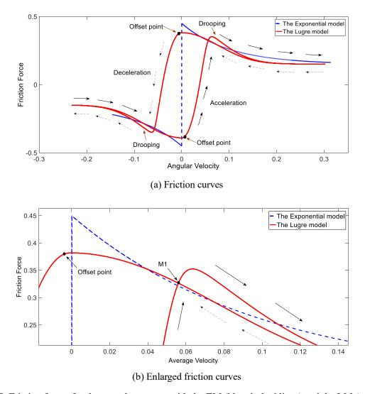
Fig. 8. Friction forces for the capsule systems with the EM (blue dashed lines) and the LM (red solid lines) show the friction characteristics near zero velocity, obtained for  $\lambda = 2.5$ ,  $\rho = 2.0$  and v = 1.0.
