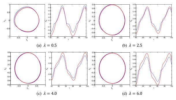
Fig. 10. Phase domain trajectories for the pendulum subsystem ( $y_1$  and  $y_2$ ) and time domain trajectories for the capsule subsystem (progressive velocity  $y_4$ ), with the LM (red solid lines) and the EM (blue dashed lines), obtained for h = 1.8,  $\omega = 1.0$ ,  $\rho = 4.0$  and v = 1.2.
