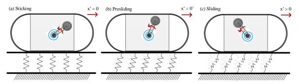
Fig. 4. Schematics of the microscopic elastic limit for the sticking, presliding and pure sliding phases.
